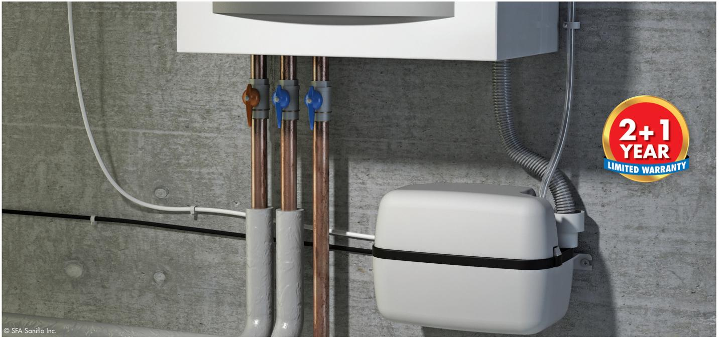
The Sanicondens is a small pump used to pump condensate from condensing boilers, HVAC systems, water heater systems, etc. The Sanicondens will pump condensate waste up to 15 feet in height and/or 150 feet away from a soil stack.
